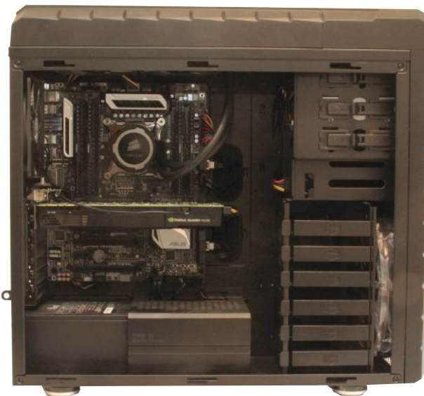
The well-organized interior of the @Xi workstation hosts an ASUS motherboard, with an over-clocked Intel Core i7 processor hidden beneath a sealed liquid cooling system and eight memory sockets, four on either side of the CPU. Images courtesy of David Cohn.
