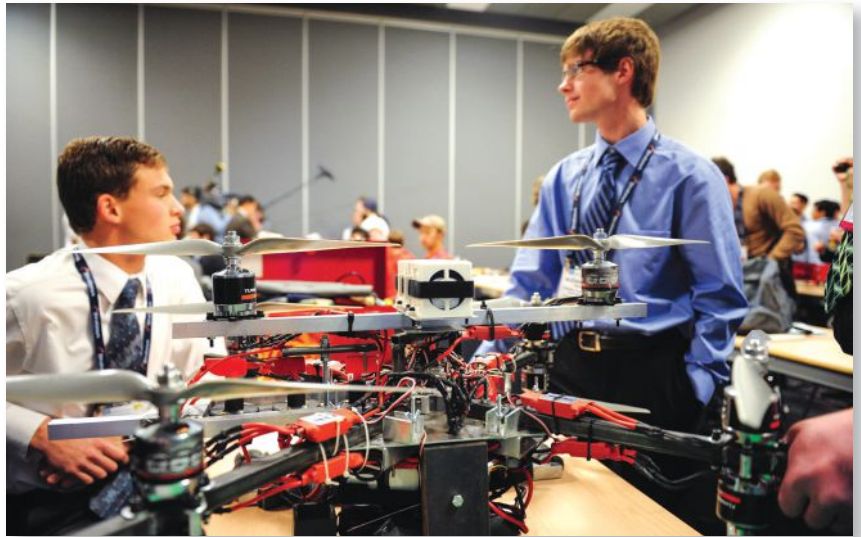
To build their UAV, the University of North Dakota team used modeling software, CNC machining and 3D printing. Image courtesy of the University of North Dakota.
