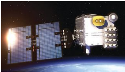
NASA's JPL is developing the antenna arrays to place on FORMOSAT-7 COSMIC-2 satellites. The mission will collect atmospheric data.
