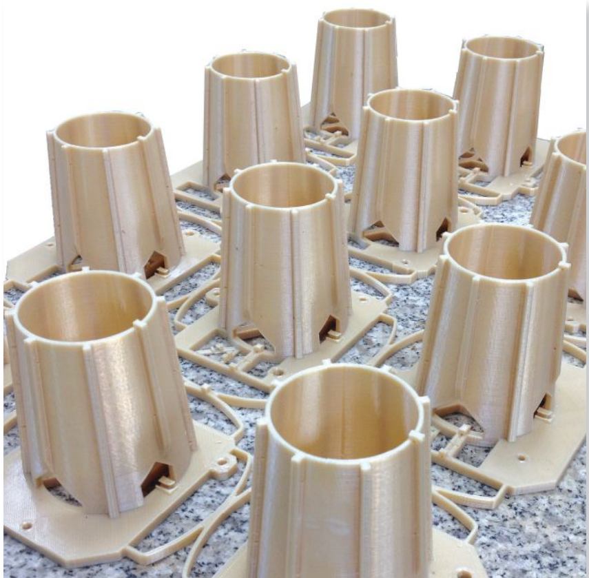
RedEye used fused deposition modeling and the ULTEM 9085 thermoplastic to create an array that matched NASA's specifications.
